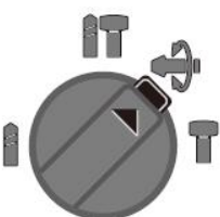
Vario-Lock position for adjustment of the chiseling position
